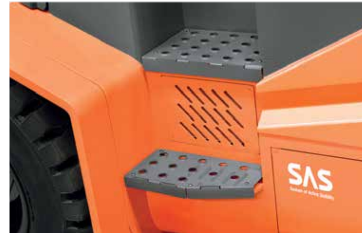
The low and wide steps and large driver assist grip ensure fatigue is minimised in applications that require repeatedly getting in and out.
