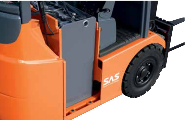
Standard low lift-out battery extraction. Built-in rollerbed for fast changes optional
