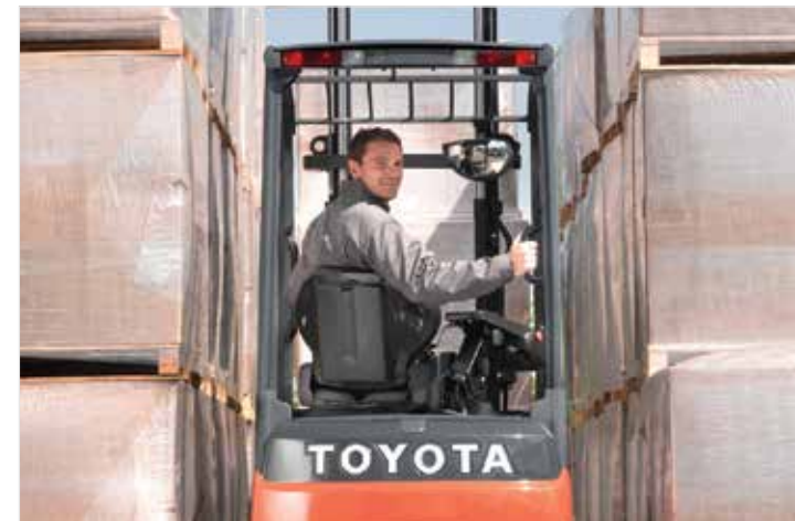
Rear-assist grip enhances reverse travel comfort and productivity by reducing operator back strain. Optional swivel seat aids comfort reversing and getting in and out
