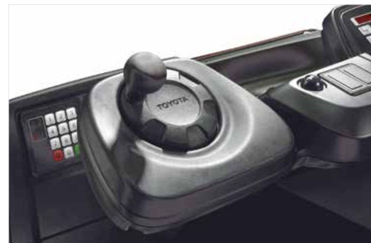
BT Reflex N-series models feature 360° steering, for intuitive and responsive control
