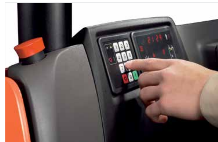
BT Access Control is standard, preventing unauthorised use
